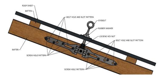
The HingeLink is designed for use on timber structures where there is easy access to the underside of the roof.
